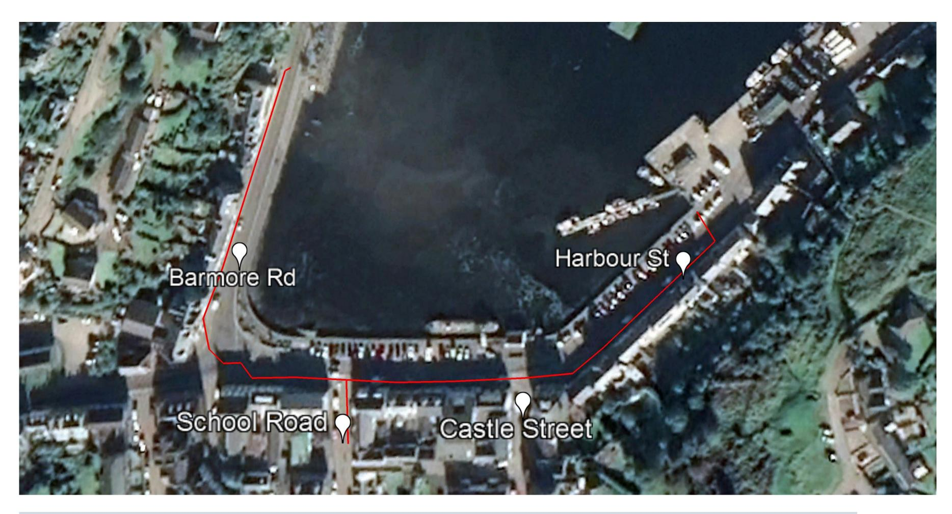
Key — = Open cut new pipes shown in Red
