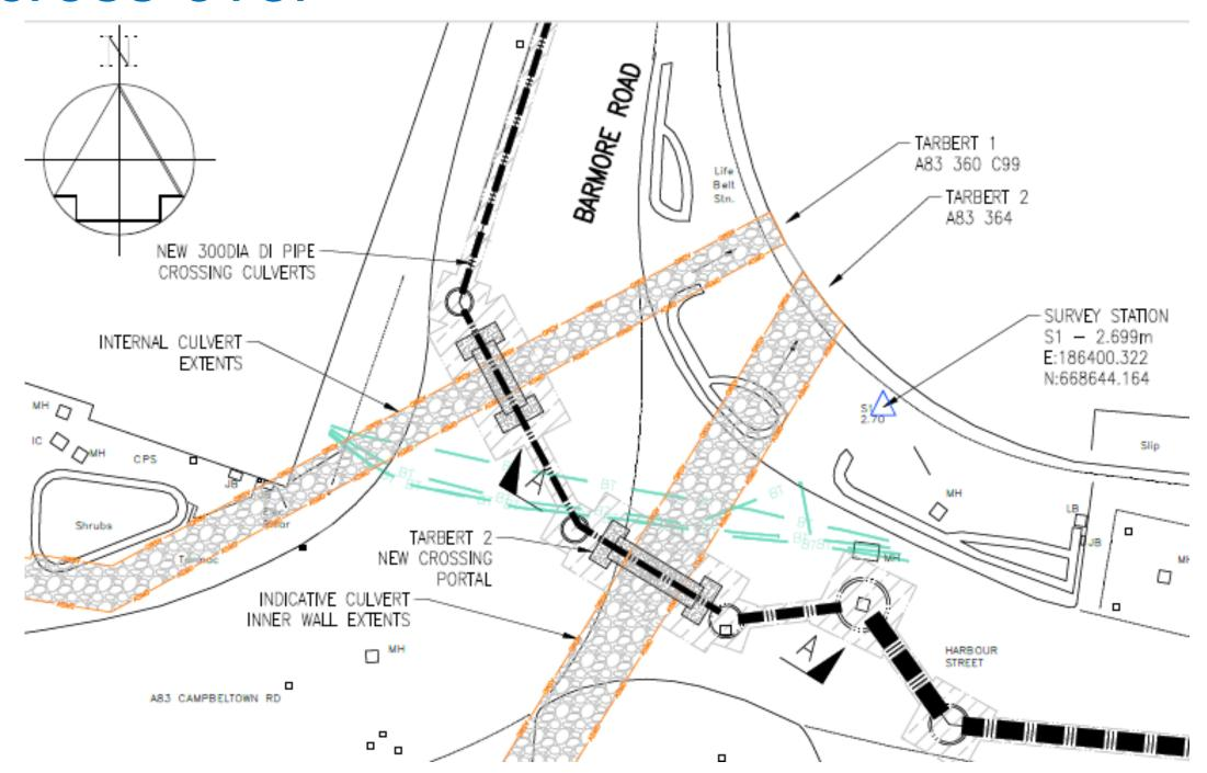
• To do this we have agreed with Traffic Scotland to construct a beam over the culvert to support the traffic while protecting the structural integrity of the culvert.
